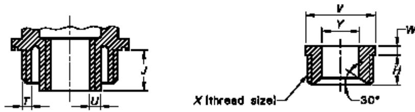
(b) Alternative section through bottom of head for DN 32 to DN 50 taps      (c) Section through gland
